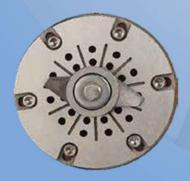
The ZEP revolutionary design features a rotating cutter bar with innovative geometry, specifically designed to address the challenges posed by stringy solids. By rotating across the strategically placed thru-holes in the cutter plate, it creates a powerful slicing action that greatly minimizes the risk of these solids rolling into the troublesome ropes and ponytails notorious for causing clogs and jams in competing products.
